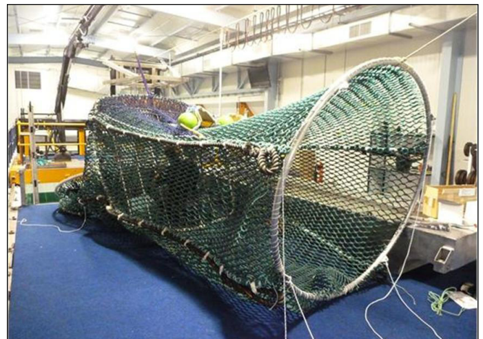
The new seal excluder device, ready to be tested in the flume tank
