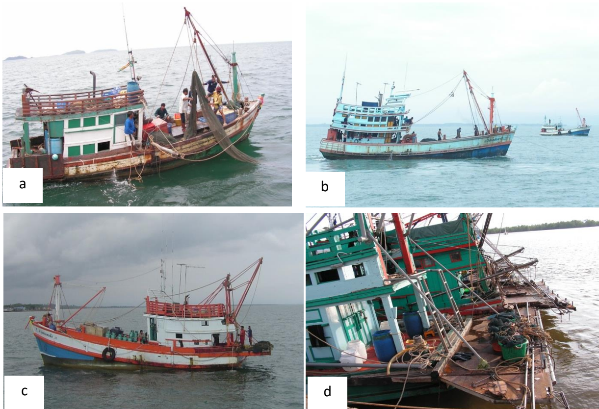
Figure 8: Trawlers in the Gulf of Thailand: a) Otter board trawler, b) Pair trawlers, c) and d) Beam trawler.
