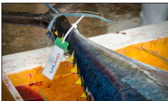
NFC Cards, like the one shown above, are used by FAME's eCDT technology to capture, store, and transmit traceability data. Photo: USAID Oceans/IF.Maruf
