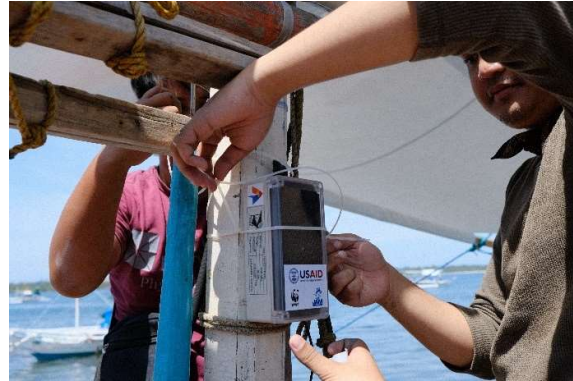
Installation of FAME transponder to a small-scale tuna handline fishing vessel. Photo: WWF-Philippines/David N. David
