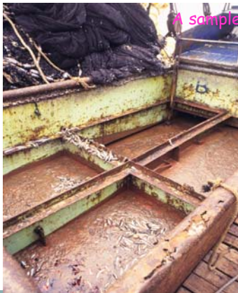
Illustrated fishes in fish hold of a purse seine. Fish is decomposing as results of lag of Cooling medium.
