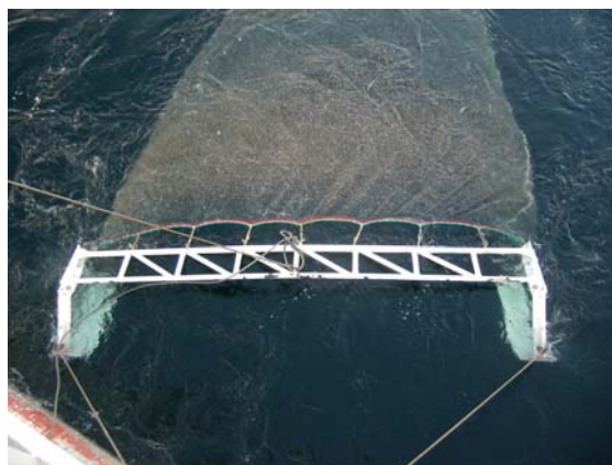
Figure 23. Fishing trials of Beam Trawl on M/V SEAFDEC2.
