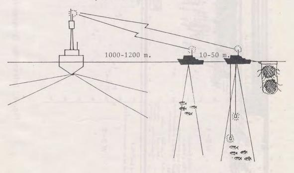
Fig. 5 Fish confirmation at PAYAO or FADs by tele-sounder
