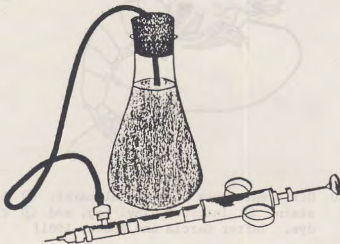
Fig. 19 Automatic injection system (from Neal, 1969, FAO)
