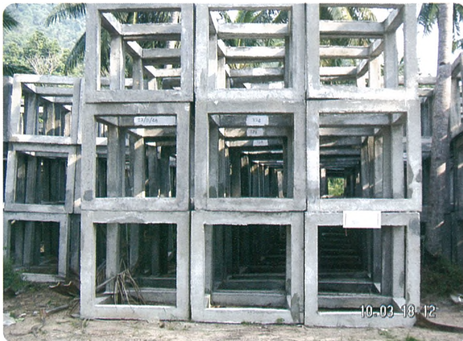
Figure 1. Concrete box type artificial reefs
