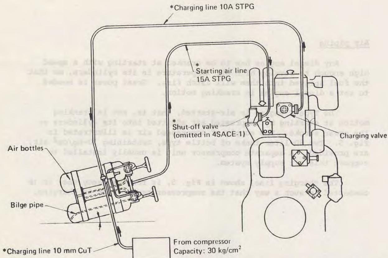
Note: Parts marked \* are meant to be installed at shipyard.
