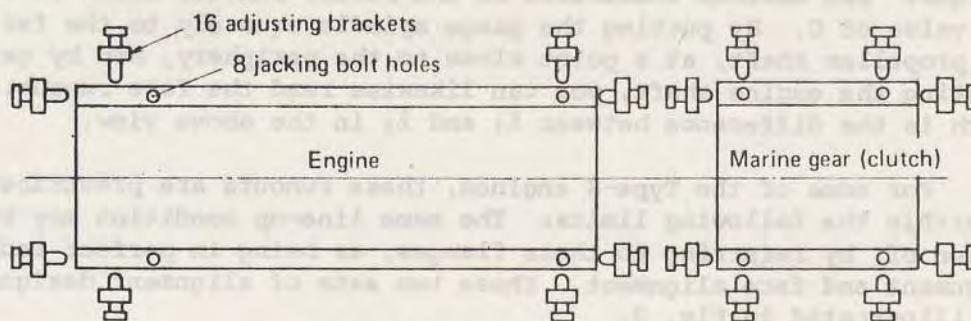
Fig. 2 Adjusting bracket positions
