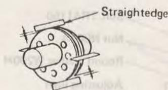
Fig. 5 Checking radial alignment
