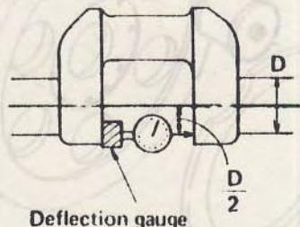
Fig. 13 Taking deflection readings at a crankpin
