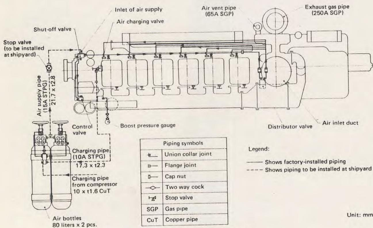
Fig. 5 Starting air piping (EY23570)
