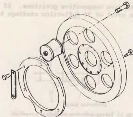
Fig. 12 Damper assembly in exploded view
