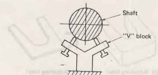
Fig. 4 Supporting a shaft for "truing up"
