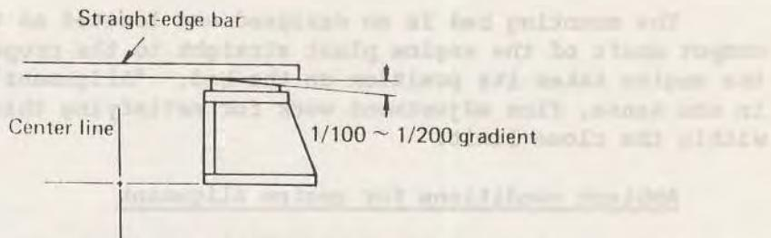
Fig. 2. Levelness and flatness of bed liners
