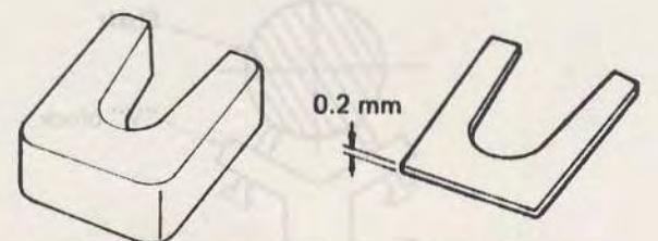
(a) Adjusting liner: TB48082 (8-piece set)      (b) Adjusting liner: TB48083 (40-piece set)
