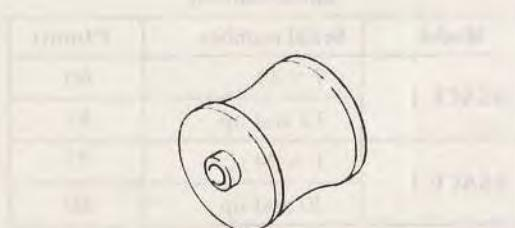
Fig. 11 Damping element of the damper
