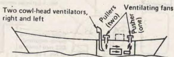
Fig. 1 Engine-room ventilation
