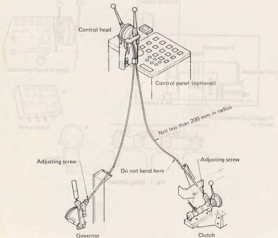
Fig. 1 Remote-control cable lines
