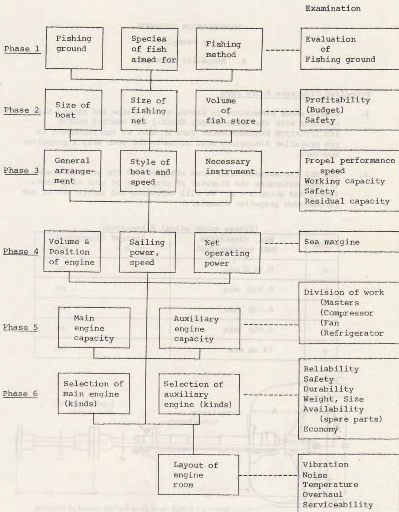
Fig. 1. The procedure in engine selection (from "Fishing Techniques", JICA, Dec. 1975)
