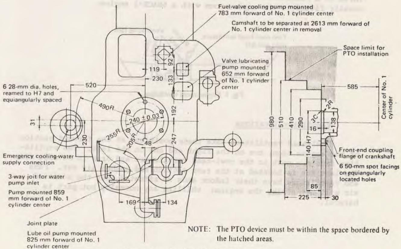
Details of front-end PTO for 6SACE-1 engine
