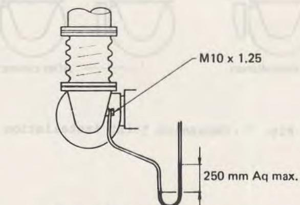
Fig. 6 Back pressure measurement
