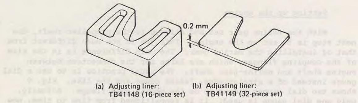
Fig. 10 Adjusting liners for the engine
