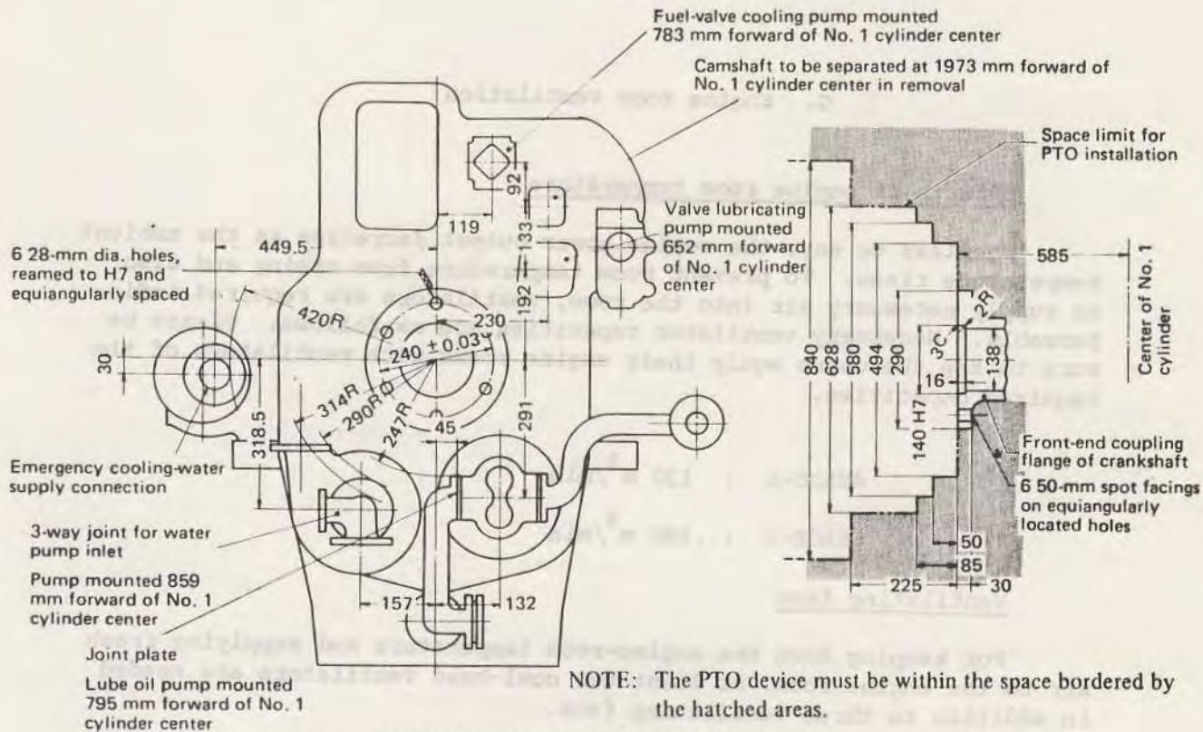
Details of front-end PTO for 4SACE-1 engine
