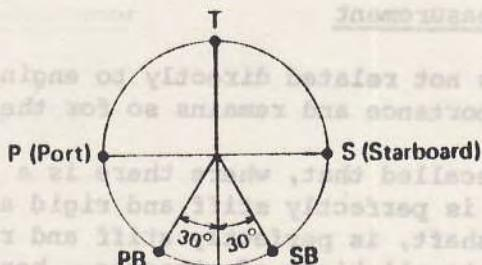
Fig. 14 Angular positions at which readings are taken
