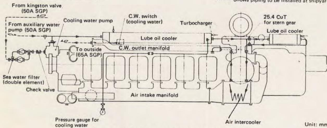
Fig. 4 Cooling water piping (EY23570)
