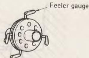
Fig. 6 Checking face alignment
