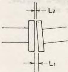
Two shafts are in perfect alignment when  $L_1 = L_2$ ,  $R_1 = 0$  and  $R_2 = 0$
