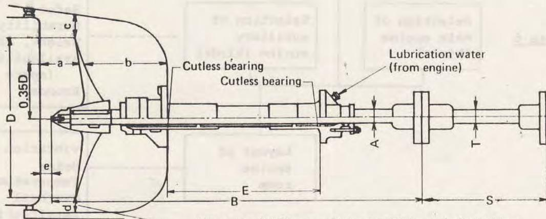
Where d = 0.06D, move Zn to the side instead of attaching it on top of shoe piece.
