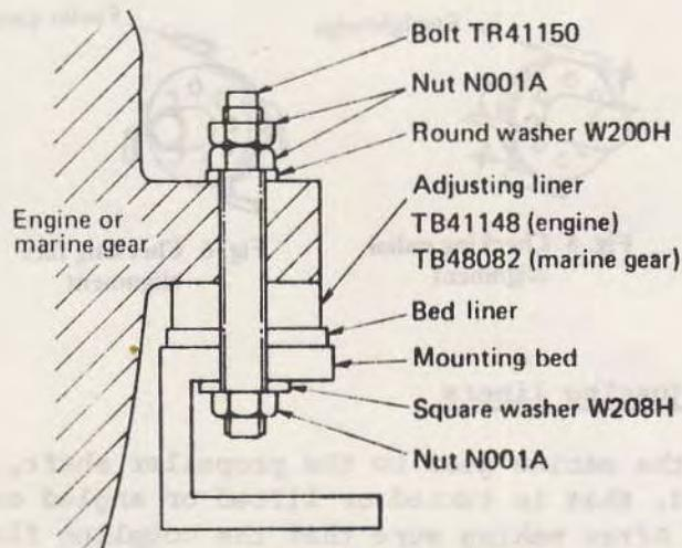
Fig. 8 Bolting to the mounting bed
