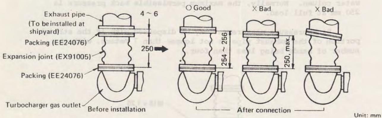
Fig. 7 Expansion joint installation
