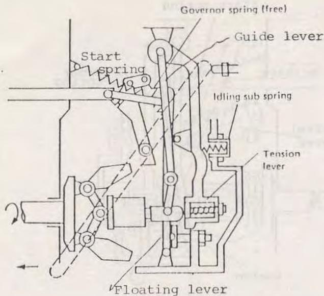
Fig. 3 Condition of the governor during idling
