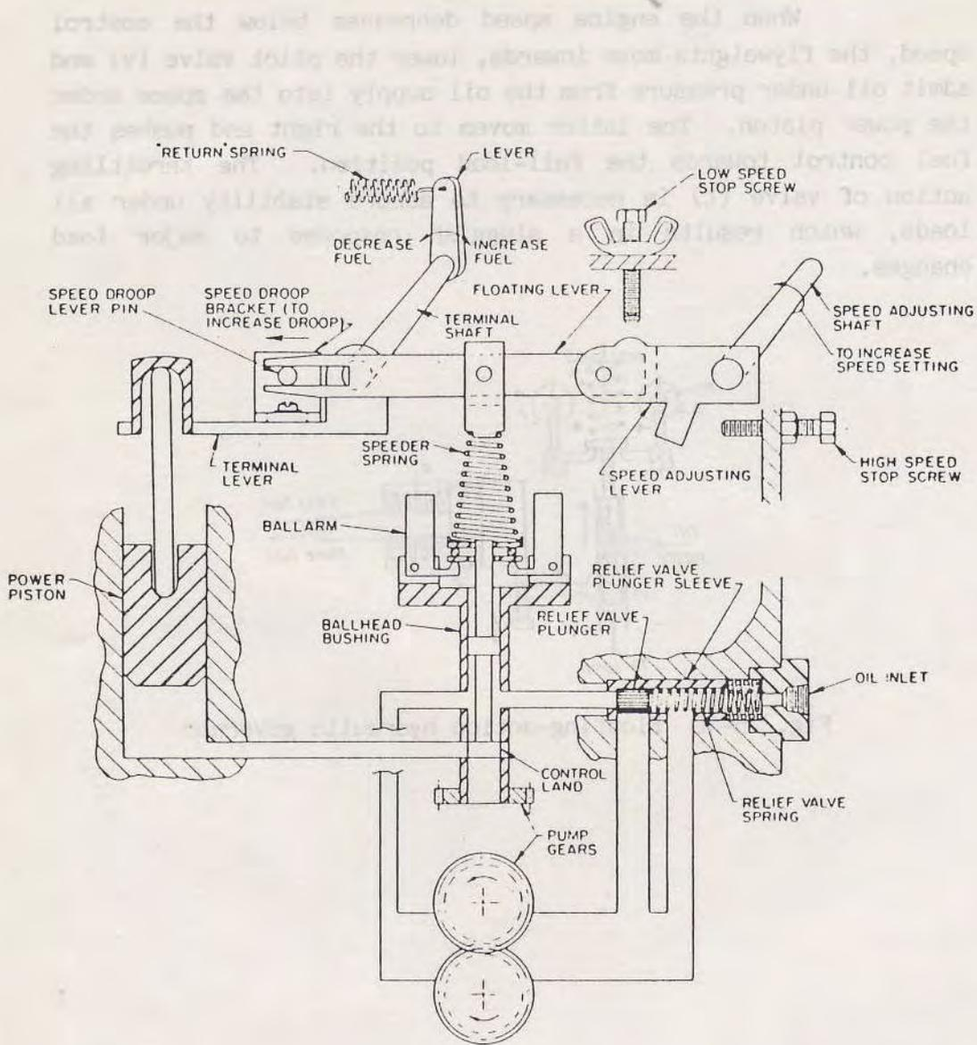
Fig. 15-11 Schematic Diagram of a Typical Hydraulic Governor
