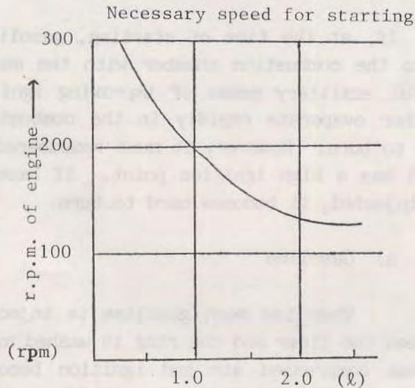
Fig. 14-5 Cylinder capacity of single cylinder
