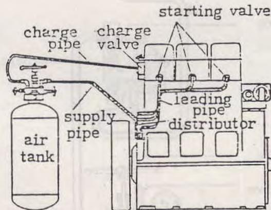
Fig. 14-8(a) Non-maneuvering valve starting system
