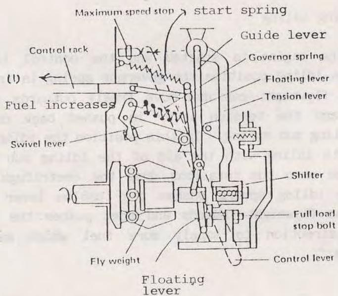
Fig. 2 Condition of the governor during engine start
