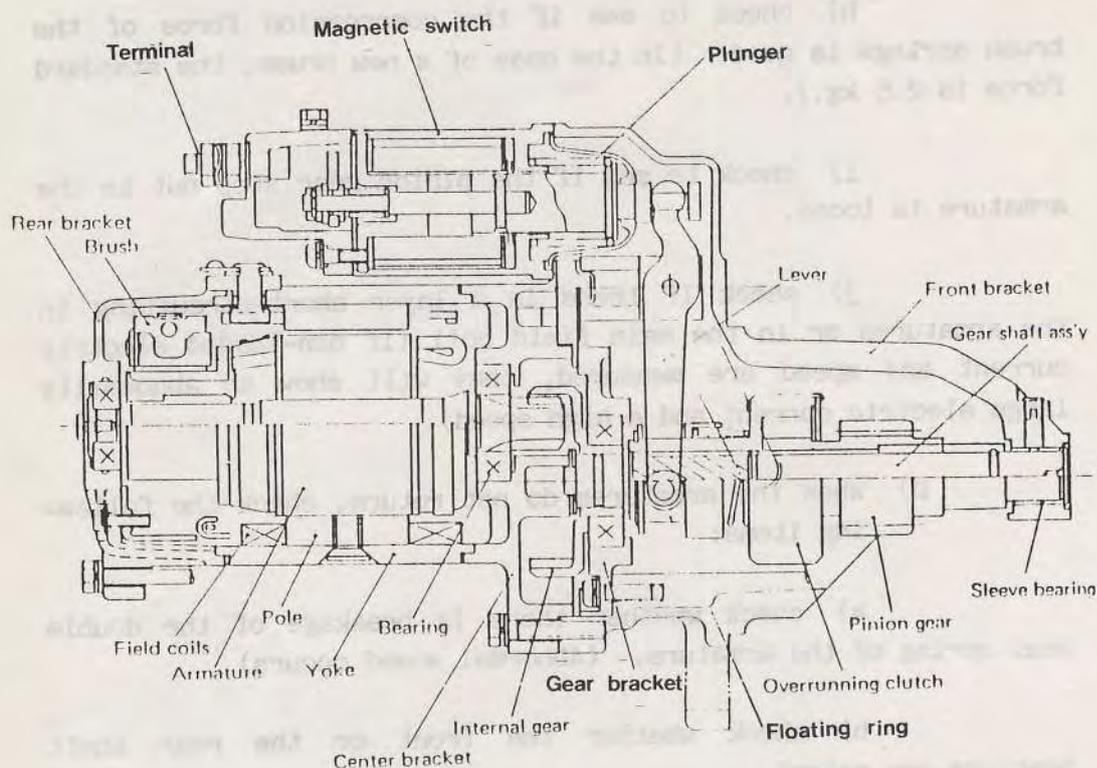
Fig. 14-39 Starter (Reduction gear type)
