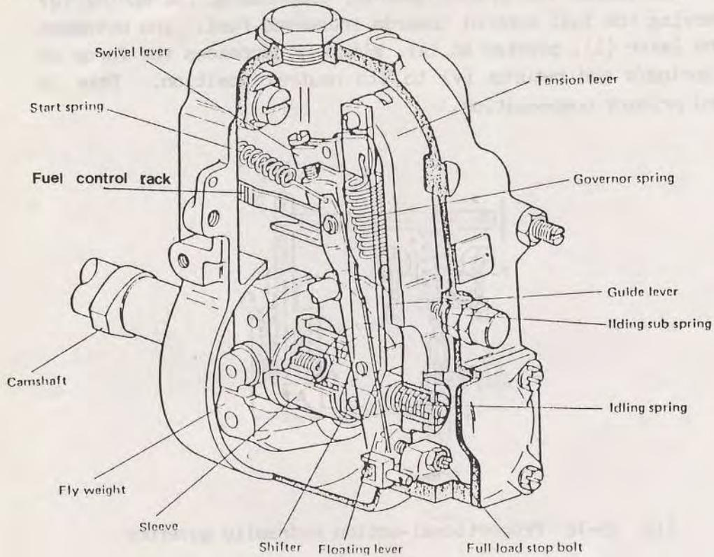
The Figure above shows the construction of a mechanical governor. The Figure below shows the various conditions according to the operating condition of this governor. Explain each step in these actions during (Fig. 1) engine stop, (Fig. 2) when engine is started, (Fig. 3) during idling and (Fig. 4) during maximum speed, respectively.
