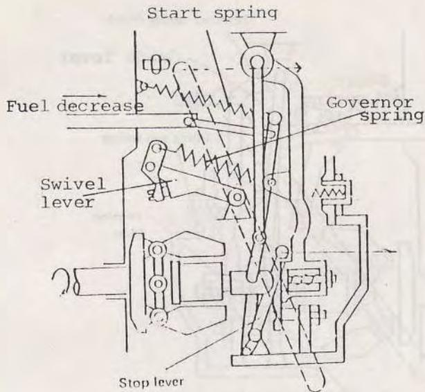
Fig. 1 Condition during engine stop
