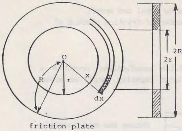
The figure shows a friction plate whose diameter is  $2R$  with the hole diameter  $2r$  (cm)
