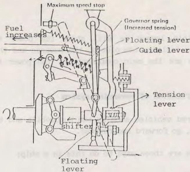
Fig. 4 Condition of the governor during maximum speed
