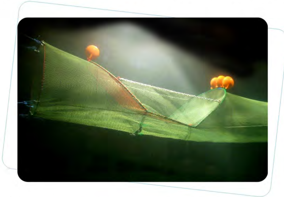
Figure 20: Buoys attached to the completed Semi-Curved Rigid Sorting Grid JTED.
