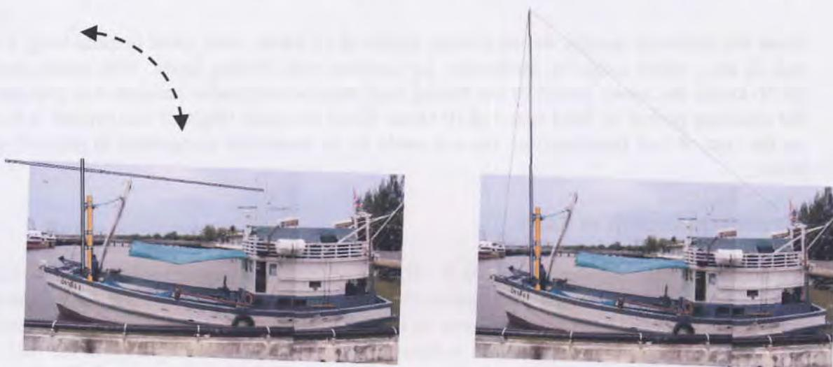
**Figure 13.** Side view of the M.V. Plalung with an auxiliary sail structure: laying down mast (left), setting up mast (right)
