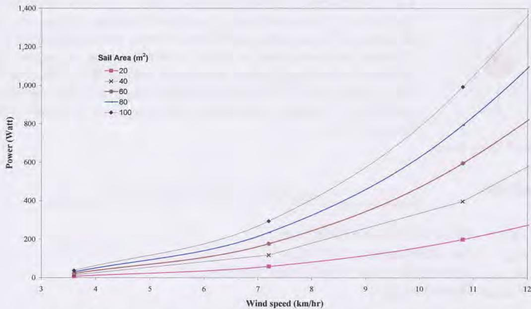
**Figure 4.** Relationship of the calculated wind power against wind speed
