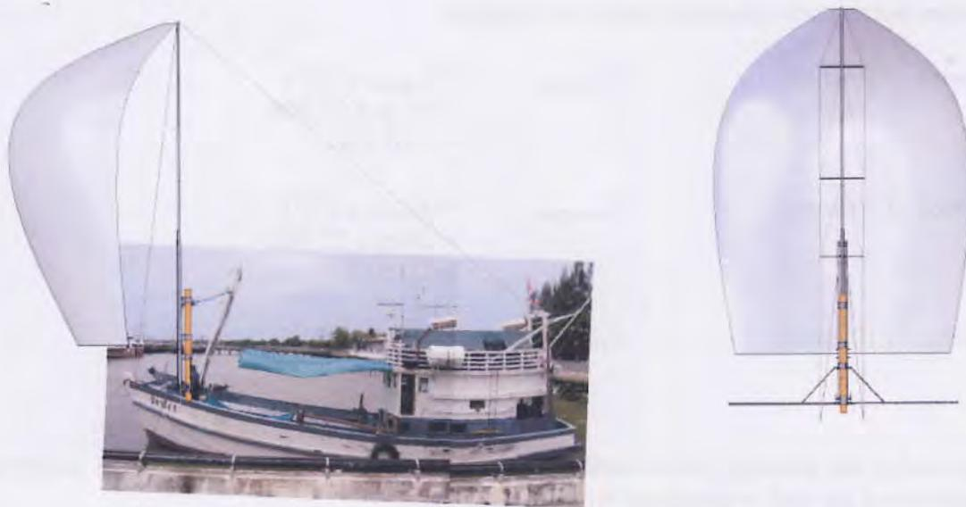
**Figure 12.** Right and front view of additional sail on M.V. Plalung
