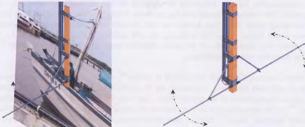
**Figure 15.** Isometric view of a side of spinnaker pole: Adjustable horizontal pole angle for directional control of sail
