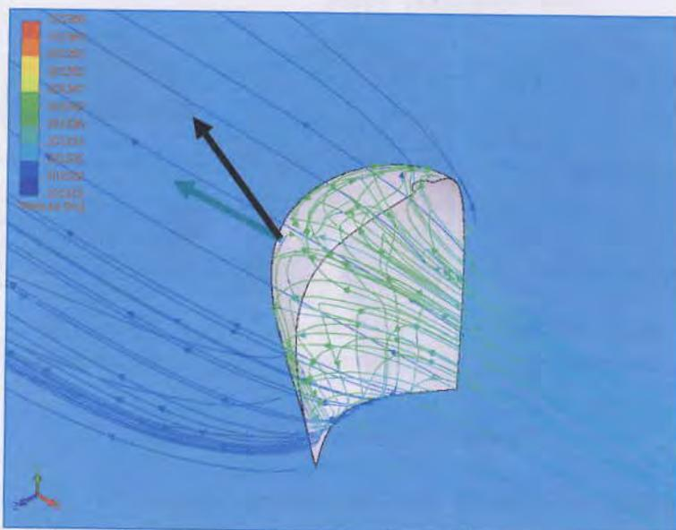
**Figure 11.** Effect of wind pressure on sail ( $105 \text{ m}^2$ ) designed for M.V. Plalung
