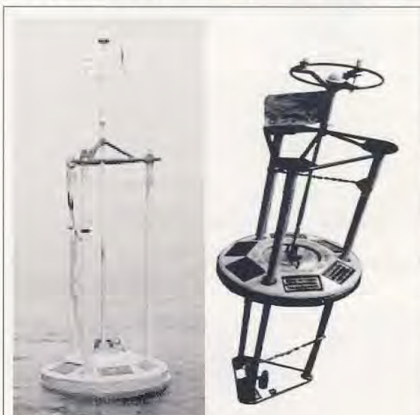
Figure 8 An oceanographic buoy was installed nearby the Set-Net for continuously data collection of weather and sea conditions at Mae Rumphueng Beach, Rayong Province
