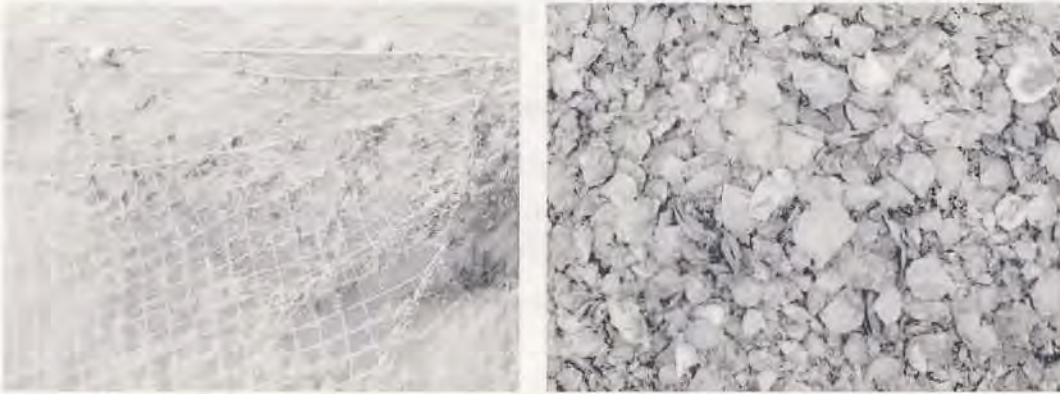
Figure 13 Settlement of sediment and organisms such as bivalves on the set-net
