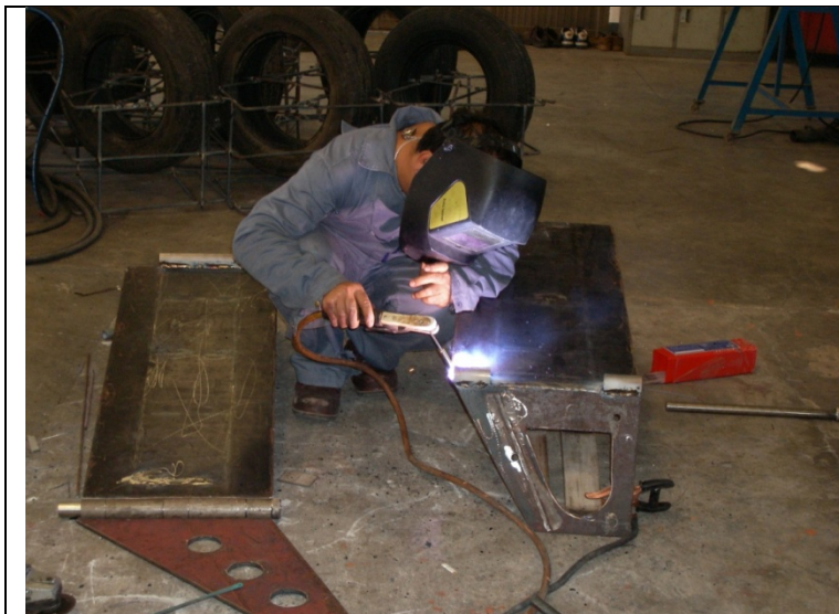
Making the depressor of the IKMT
