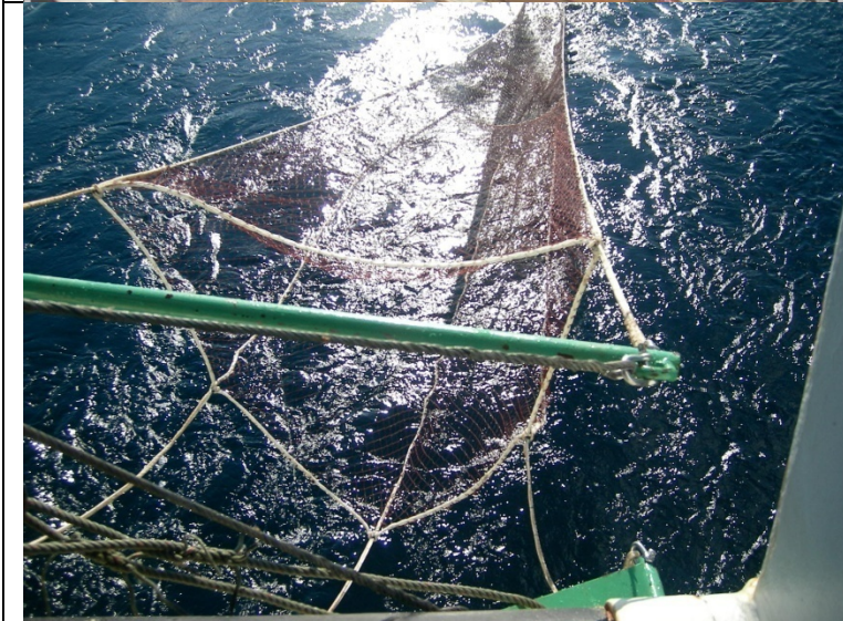
Fishing trials of IKMT on MV SEAFDEC2, Trawl net part.
