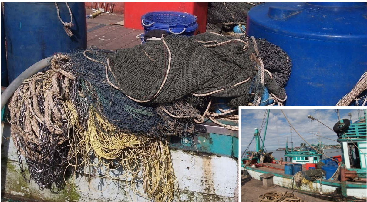
Figure14 Otter board trawl net on trawler size 14-18 m length overall (LOA) at Kor Kasemsiri fishing port Klongyai, Trat Province
