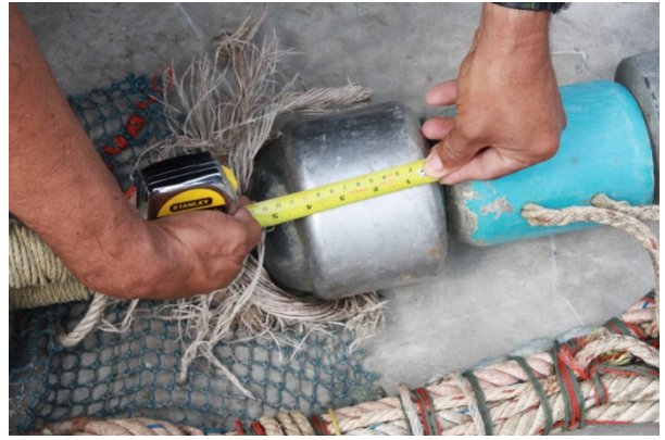
Figure 21 Wooden, rubber and stainless steel bobbin of pair trawl are assembled at ground rope
