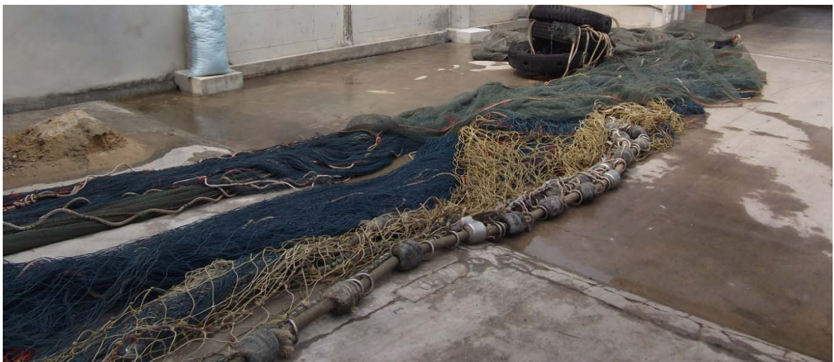
Figure 23 Wooden, rubber and stainless steel bobbin of pair trawl are assembled at ground rope
