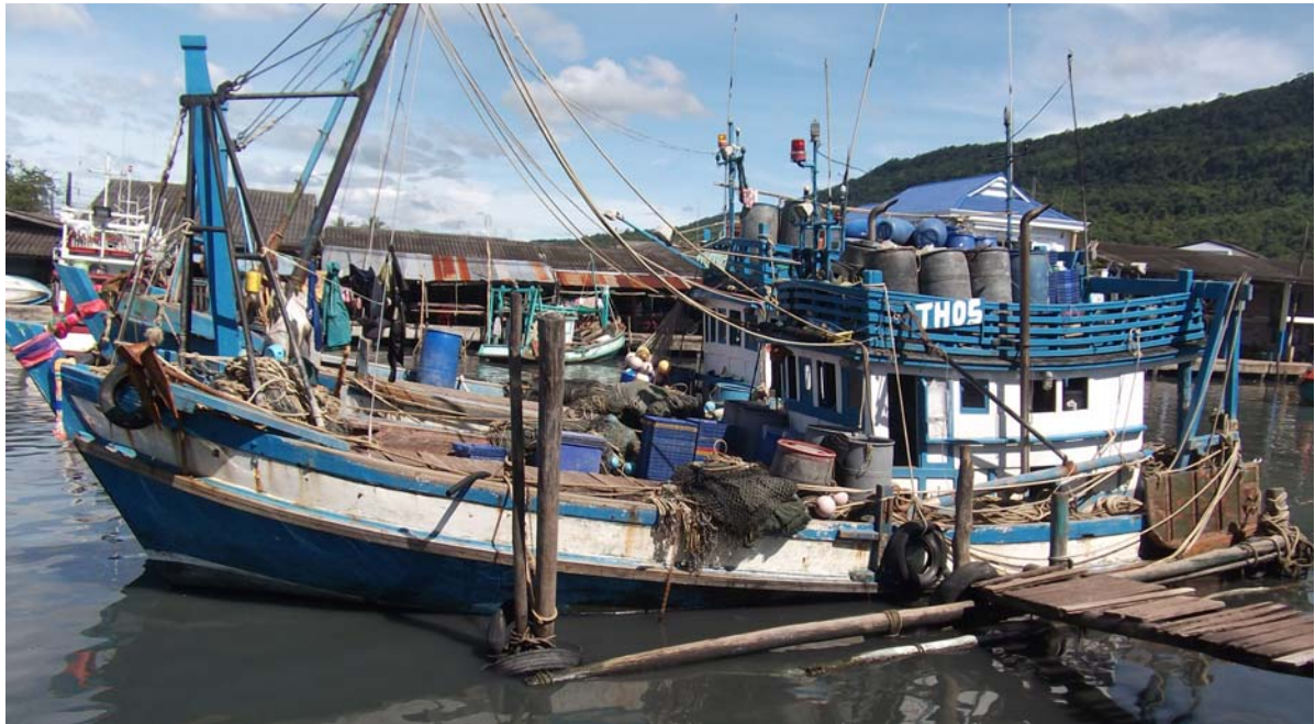
Figure12 Otter board trawler size 14-18 m length overall (LOA) at Kor Kasemsiri fishing port Klongyai, Trat Province
