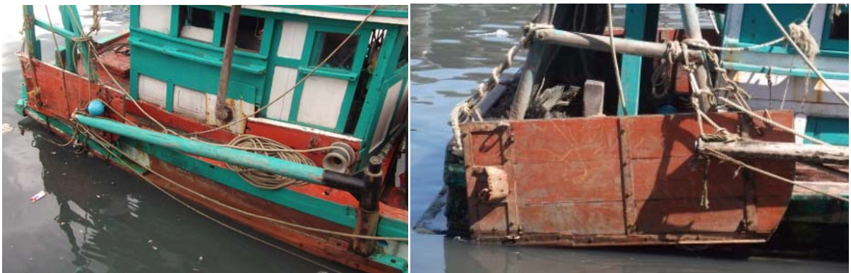
Figure 7 (Right) Trawler boom with otter board (Left) Otter board
