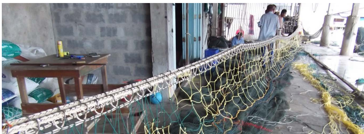
Figure 9 Selvage net of bottom wing part constructed at Fishing workshop, Klongyai, Trat Province
