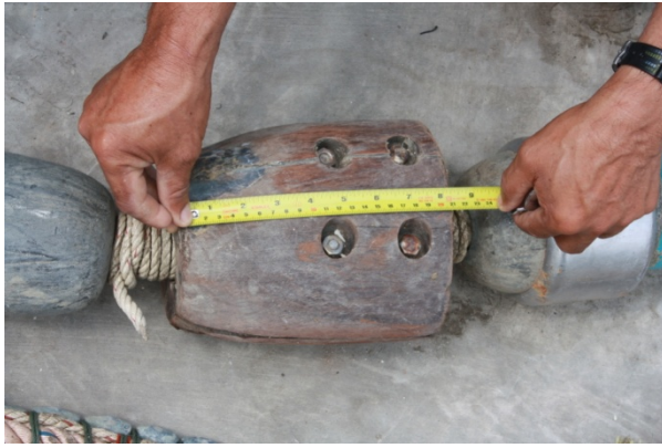
Figure 21 Wooden, rubber and stainless steel bobbin of pair trawl are assembled at ground rope
