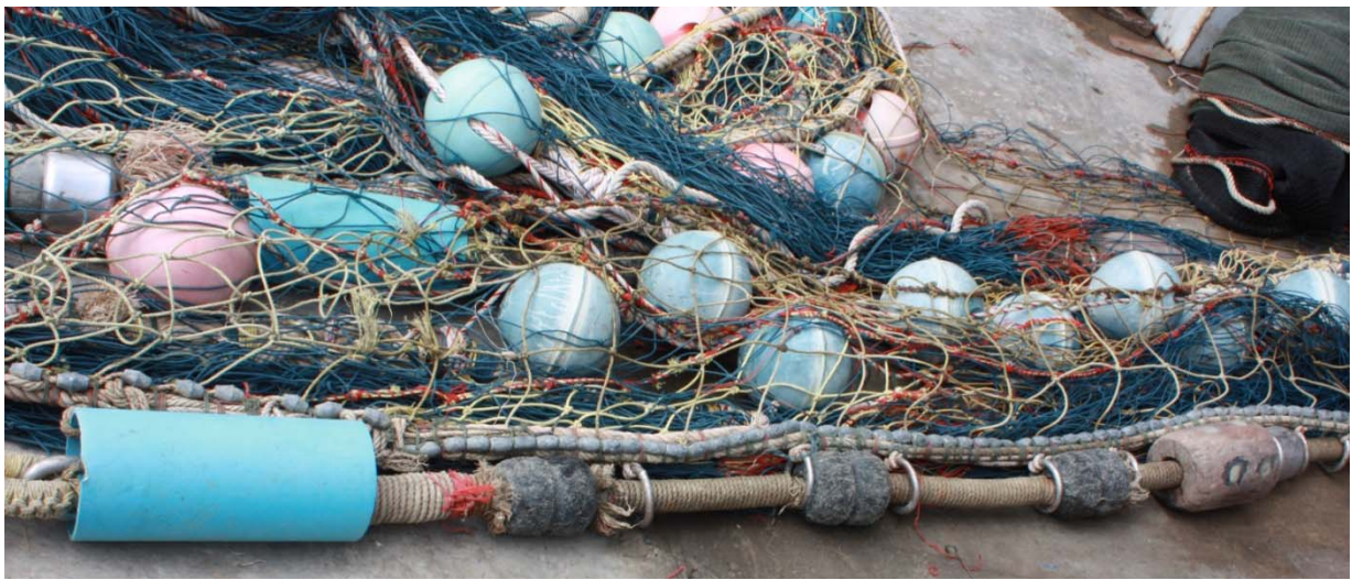
Figure 22 Ground rope, salvage net, wing net and net body of trawl net
