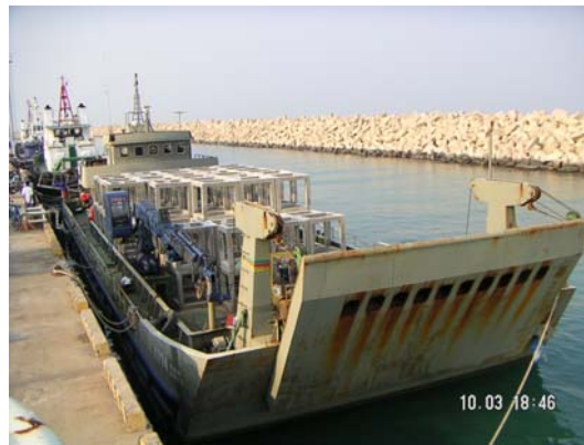
Figure 5. M.V. Khaow Khang, carry cubical shape concrete, artificial reefs to install at Pratew dis-
