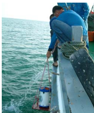
Figure 14. The water current observation was conducted by using Acoustic Doppler Current Profilers (ADCP)
