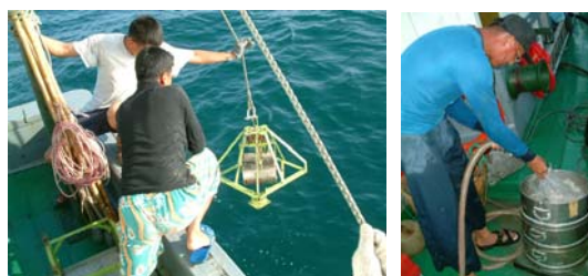
Figure 12. Random sampling of benthos by Smith-McIntyre grab and washed through a set of sieves.
