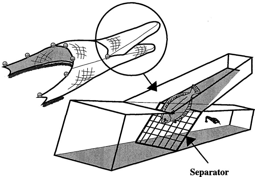
Fig.5 Basic BRD for coastal trawlers in Japan
