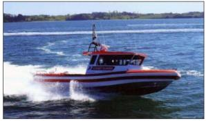
Three rescue boats had been designed by Naiad, building on their long experience both with rescue boats and jets in a variety of commercial and military applications. The key design objective has been to deliver a twin diesel jet in an economical package but still with plenty of working cockpit space, a large lock-up cabin with proper seats for four crew, forward cabin for
