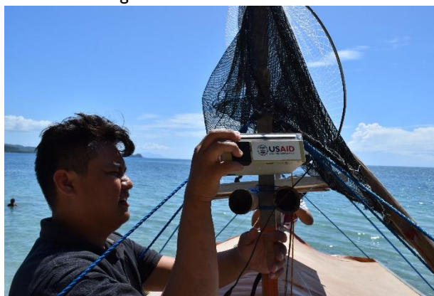
FAME staff installing transponders equip with NFC readers on small-scale vessels. Credit: USAID Oceans/L Bader
