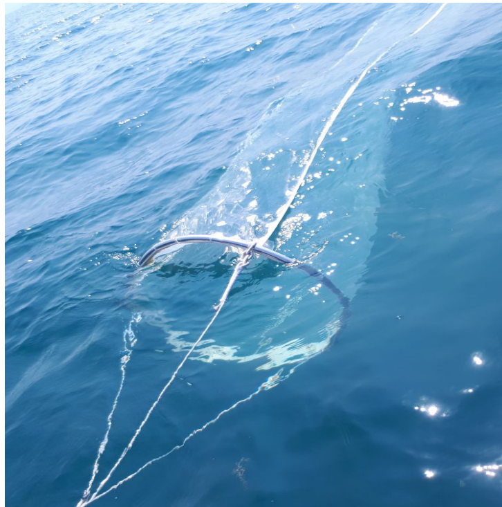
Figure 2 : Bongo net for sampling marine fish larvae
