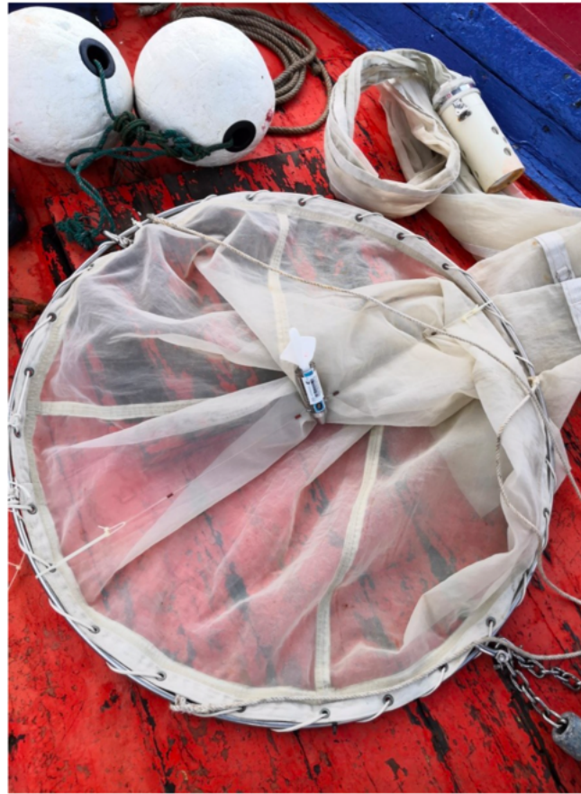
Figure 2: Sampling was conducted using a larvae net with 500 µm mesh size and a flowmeter installed to measure the flow rate of the seawater into the net
