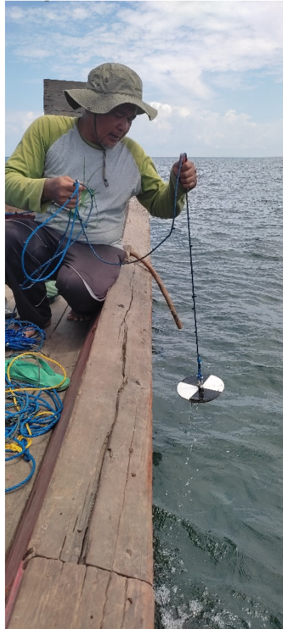
The water brightness measurement using sechi disk
