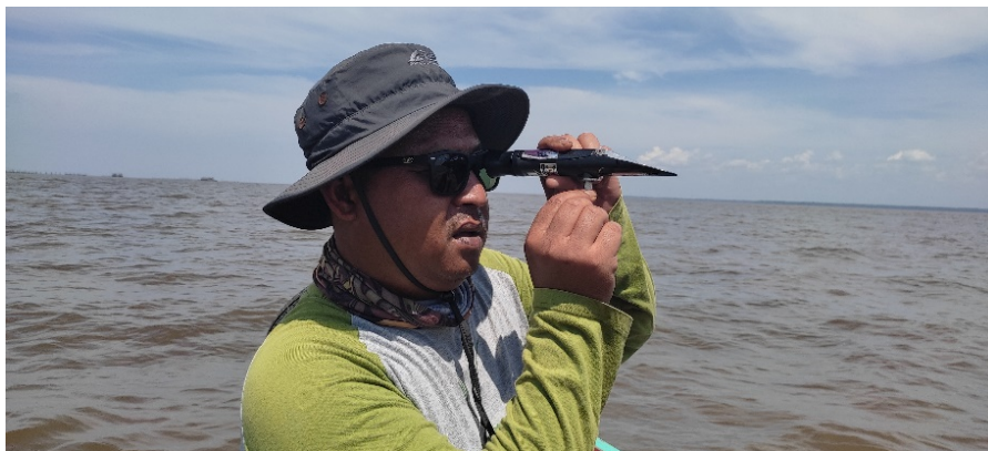
The salinity concentration measurement using refractometer
