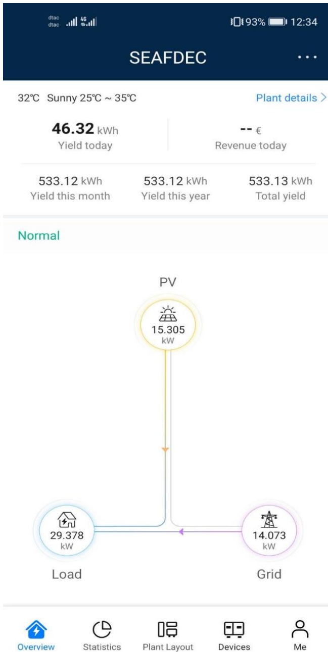
Illustrate 16. (Example 3) On-grid Solar Roof systems can observed in real-time working conditions via mobile phone.
