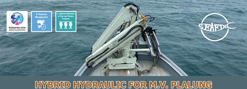
Hybrid hydraulic Systems have features that are beneficial to the operation of fishing vessels at present. The Hybrid hydraulic system launching for training and research vessel namely M.V. Plalung is providing with two-energy source consisting of a source main engine and an electric motor to produce hydraulic power source delivers to the auxiliary fishery and hauling devices onboard to have a variety of users.
