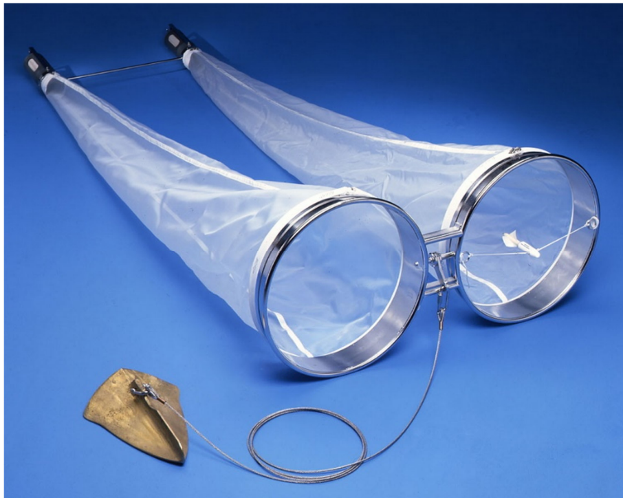
Figure 7: A 60 cm diameter Bongo net with depressor and attached flowmeter
