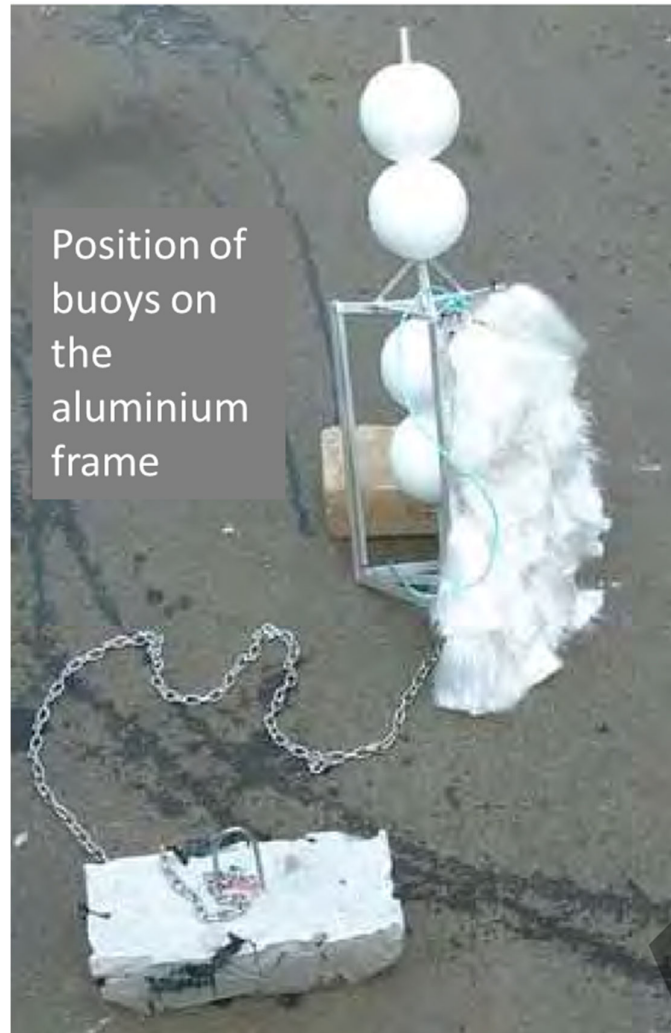
Figure 2: Frame design without PVC panel to show the inner construction of the puerulus trap (de Lestang et al., 2011)
