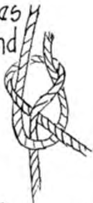
Sheet bend, double sheet bend
