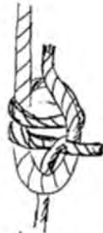
Sheet bend, double sheet bend
