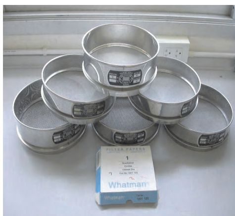
Fig.4 The series of sieve mesh size 2, 1, 0.5, 0.25, 0.125, 0.063 mm. and filter paper (whatman no.1)
