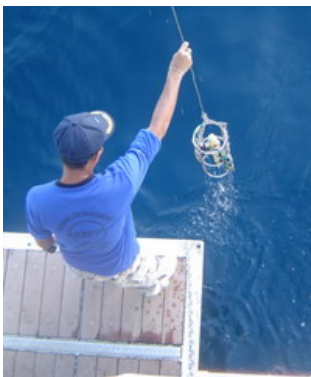
Fig. 3 STD/CTD model SD204 operation
