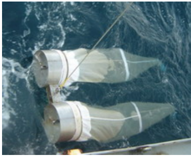
Fig.1 Bongo net operation
