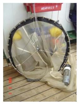
Fish larvae was sampled by fish larvae net (100 cm. in diameters) with the towing speed at 2 knot for about 15 minute in horizontal direction at surface level. The flow meters were attached at center for estimated water volume that flow passed into the nets. The fish larvae collected was preserved with 10% buffered formalin in seawater immediately. For logsheet of fish larvae operations were shown in table no. 3.1 and 3.2
