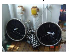
At each station a 10-15 minutes oblique tow of the bongo net was made with the ship speed 2-2.5 knots approximately. The depth of haul was 10-20 maters above the sea bottom or 85-100 meters for the station which was too deep. The samples were preserved in 10% buffered formalin and seawater immediately. For logsheet of bongo net operations were shown in table no. 2.1 and 2.2
