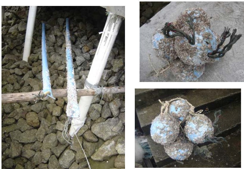
Figure 3. Marked PVC pipe and buoyancy float of FEDs were cut by commercial trawler.
