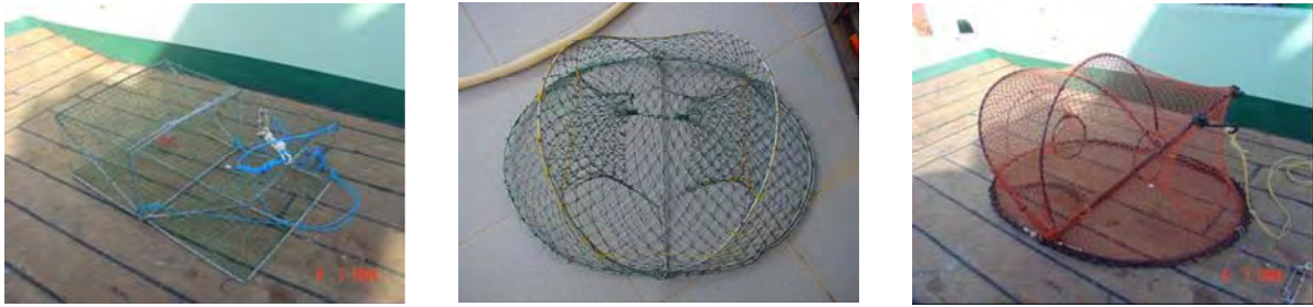
Three types of collapsible fish traps tried in Langkawi Island (Photo by Research Division, SEAFDEC/TD)
