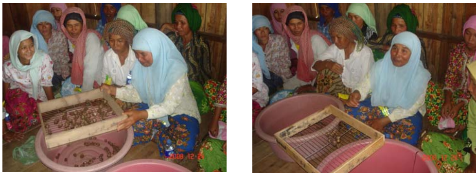
Fig. 6 Member of blood cockle fishing group tested mesh size of sieve (1.8 cm)
