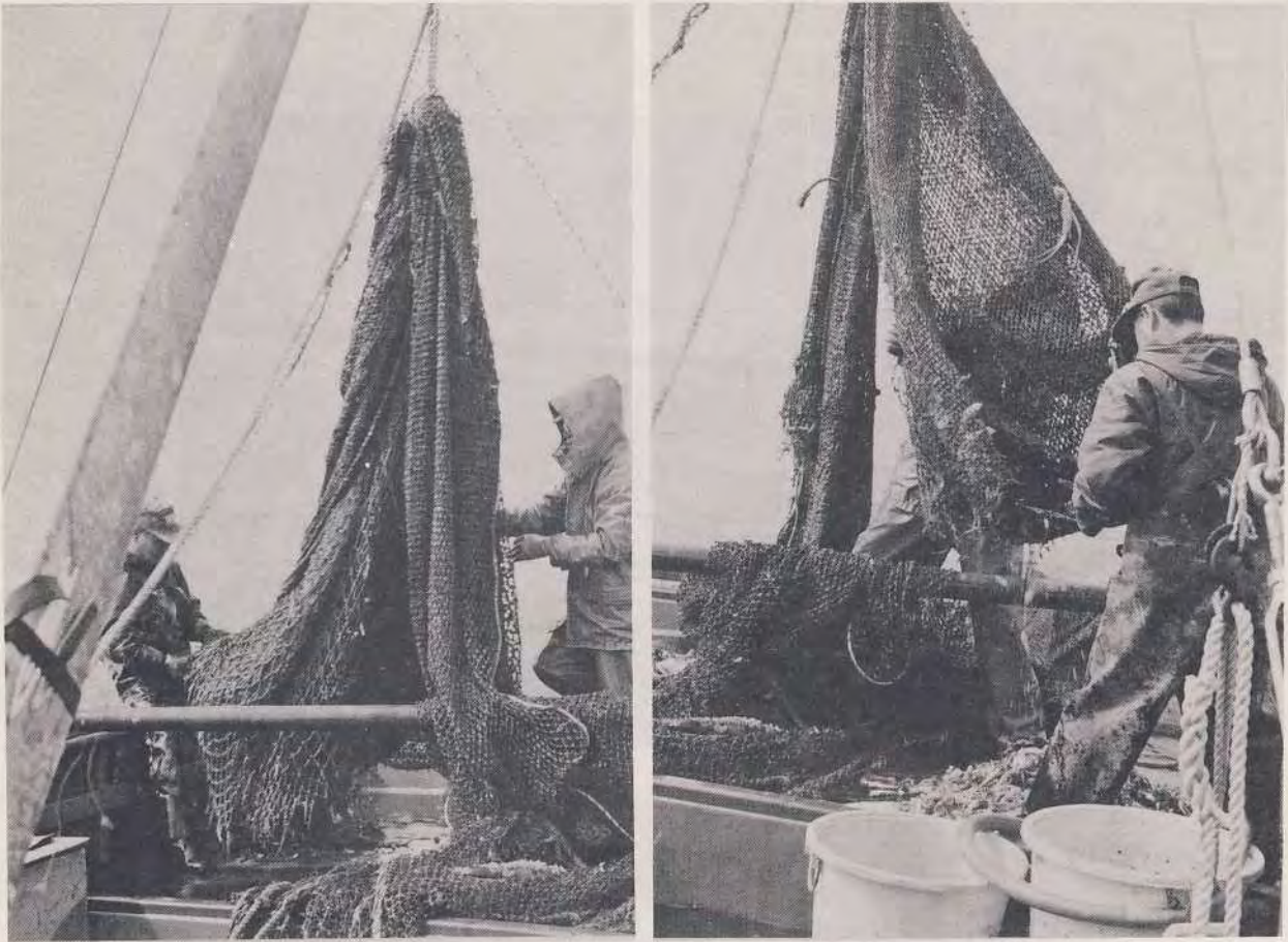
Figs. 11-12 During the hauling operation, the first and second cod end are opened.
