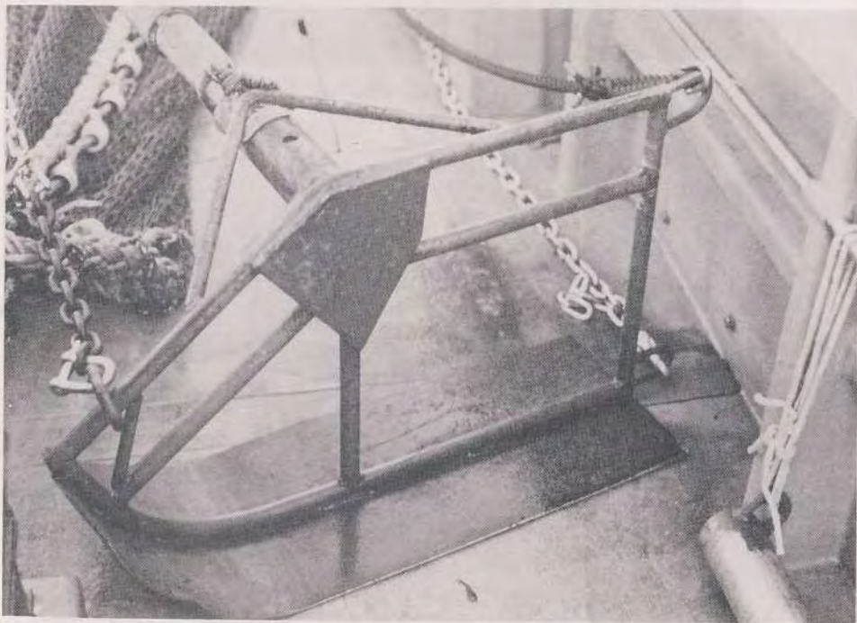
Figs. 5-6 Iron beam pipe with ski.
