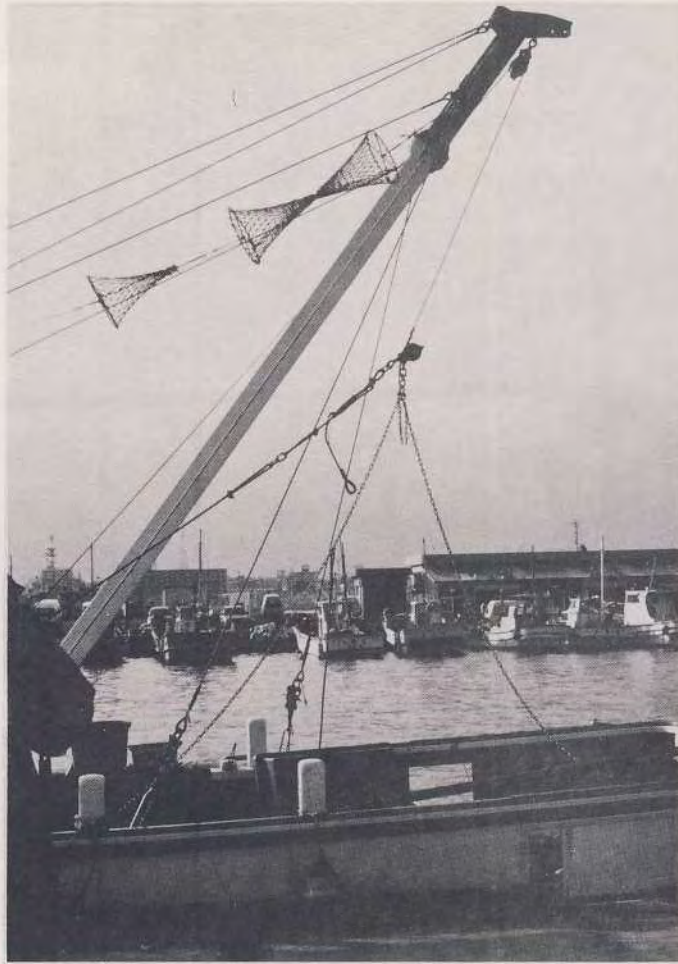
Fig. 3 Stern iron beam with pulley.
