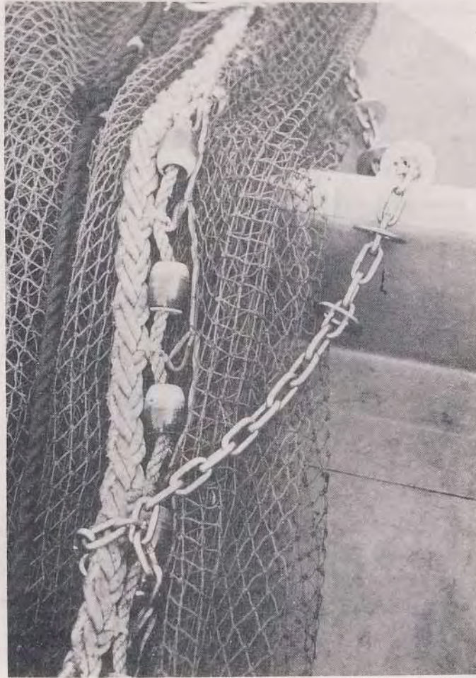
Fig. 7 Round-shape stainless plates with chains are attached to the front of the ground rope.
