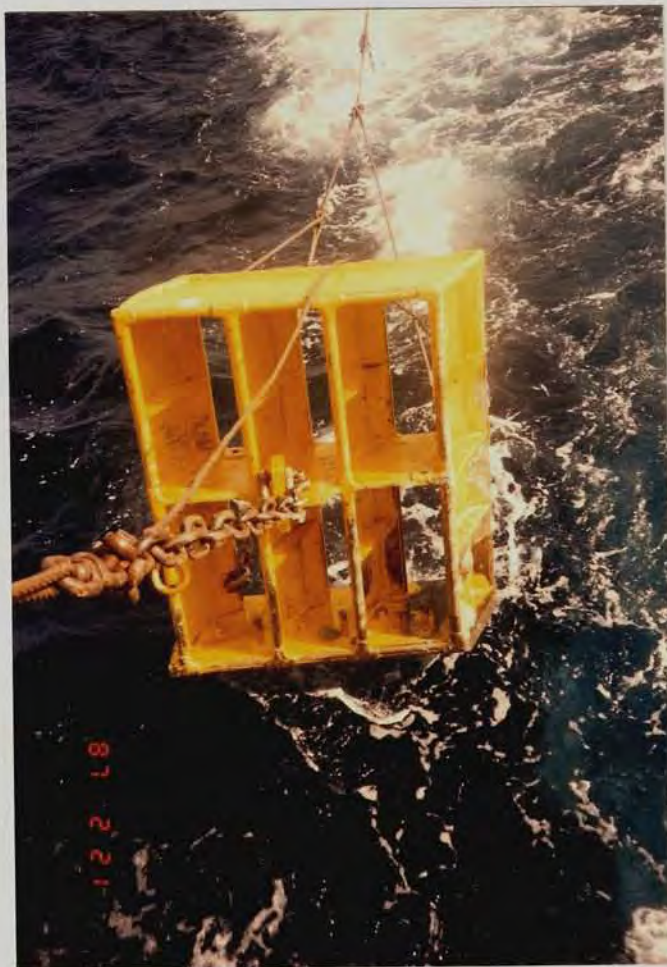
Photo. 6 Paravane otter-board shooting from M.V. PAKNAM
