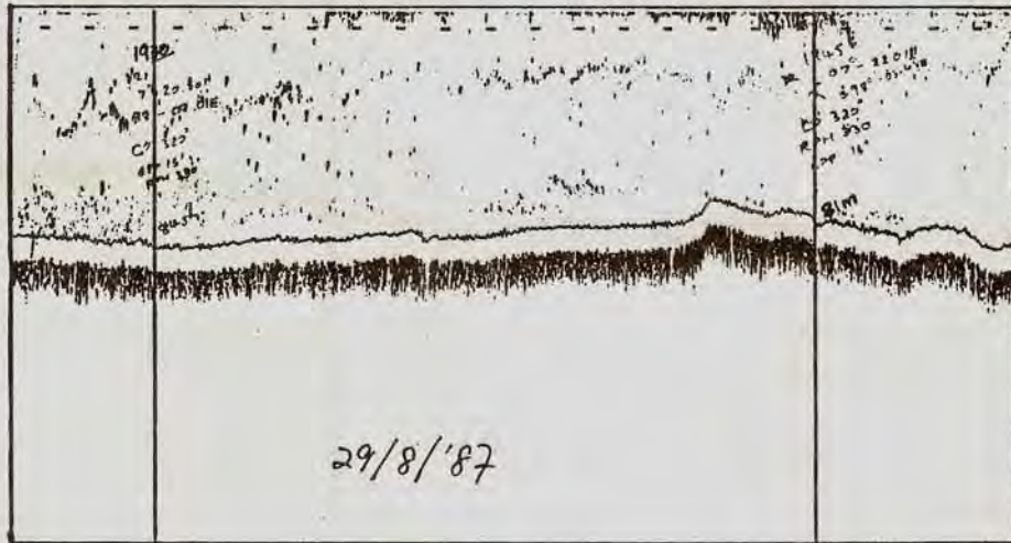
Fig. 40 Recording of sea-bed Rough, at a depth of 81 to 84 metres.
