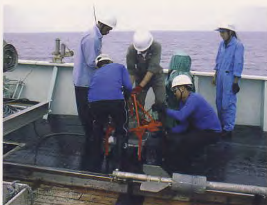
Plate 4. Smith-McIntyre Bottom-Grab and Gravity Sediment Corer [in front].
