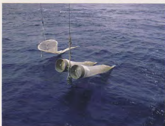
Plate 5. Fish larvae net (left) and Bongo net (right).
