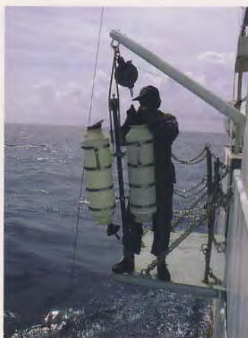
Plate 3. van Dorn Water Sampler.
