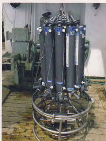
Plate 2. ICTD Unit with Rosette Water Sampler.
