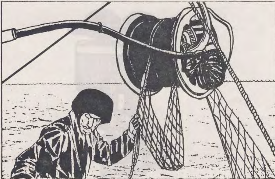
Fig. 108 A fisherman hauling gill net with a Mini Block mounted on the stern deck of his boat
