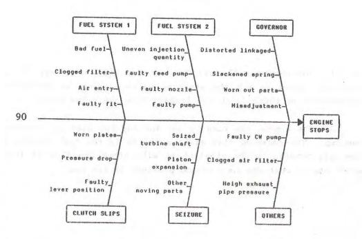
88. 3) When the engine starts but does not continue running, the cause may be found in the governor or the fuel systems, e.g. air in fuel, a clogged filter or malfunctioning injection pump.
