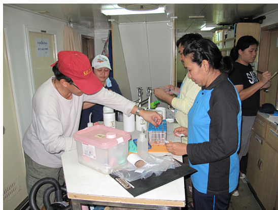
Figure 4. Water sample filtering through Whatman GFC filter paper and stored in the freezer at -45 °C for nutrient analysis.
