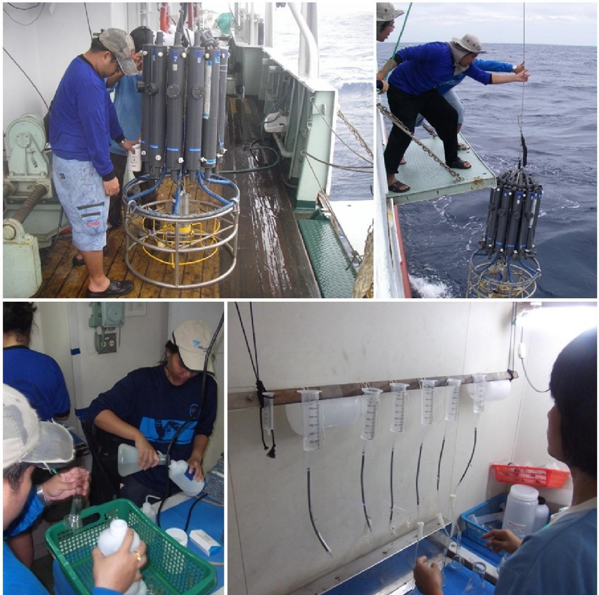
Fig.2 CTD data collection and sea water chemical analysis
