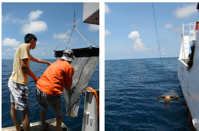
Figure 3. Neuston net towing at the sea surface.
