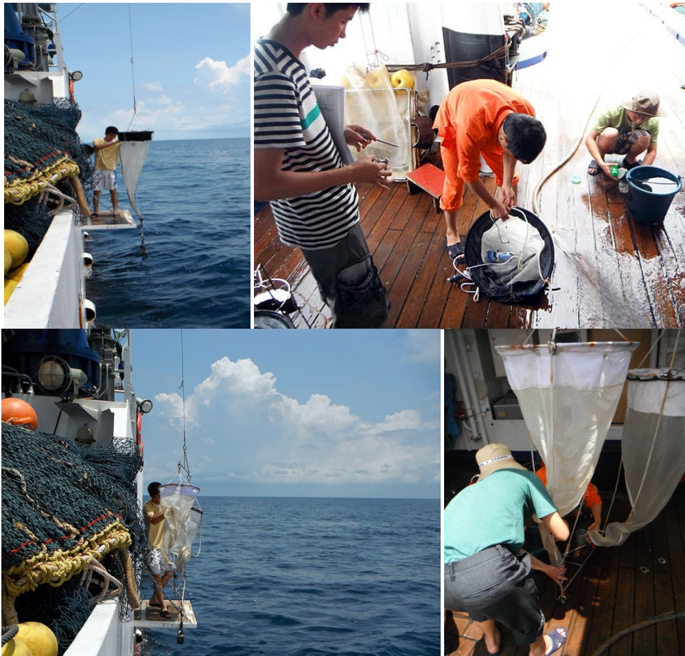
Figure 4. Vertical tow of zoo-phytoplankton net, and larvae and egg net.
