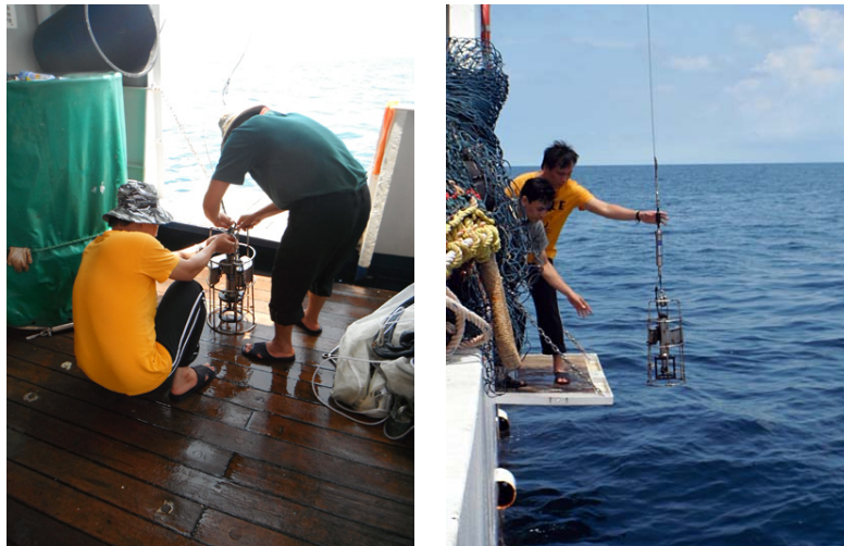
Figure 2. Compact CTD data logger and current meter deployment.
