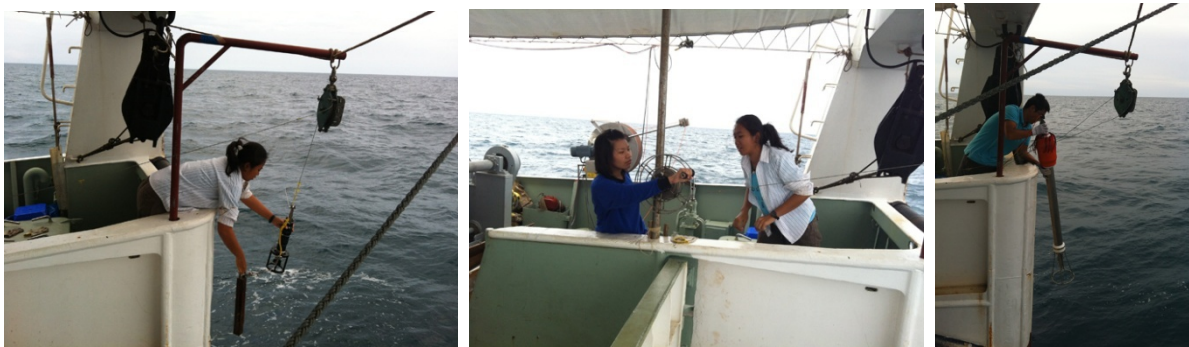
Figure 6. Compact CTD data logger and MSS90 deploy at mooring station.
