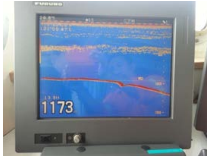
Figure 3: Monitor is one of the major components using in Scientific Echo Sounder FQ80-M System
