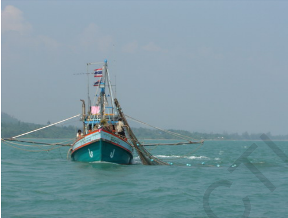
Figure 5. Otter-boom trawler usually targeting for shrimp, is hauling (LOA 14-18 m).
