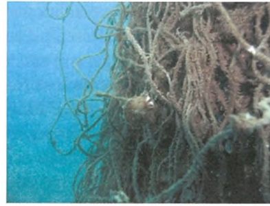
Fig. 35 Marine growth attached on FEDs appendage two month after installation
