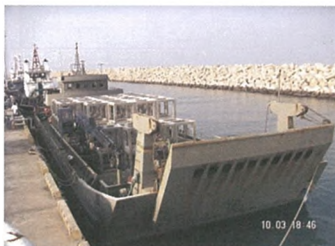
Fig. 5 M.V. Khaow Khang, carry cubical shape concrete, artificial reefs to install at Pathew District, Chumphon Province
