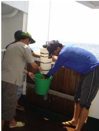
Fig. 6 Collect large volume of water sample using Van Dorn water sample
