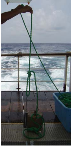
Fig 7. Temperature and Depth recorder attached with BVL
