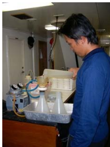
Fig. 5 Water filtering for TSS.
