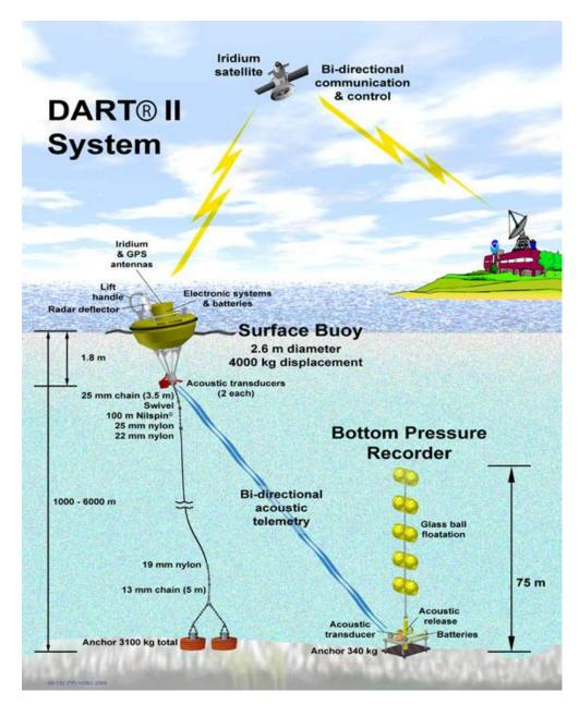
Installation system DART II is composed of two parts.
