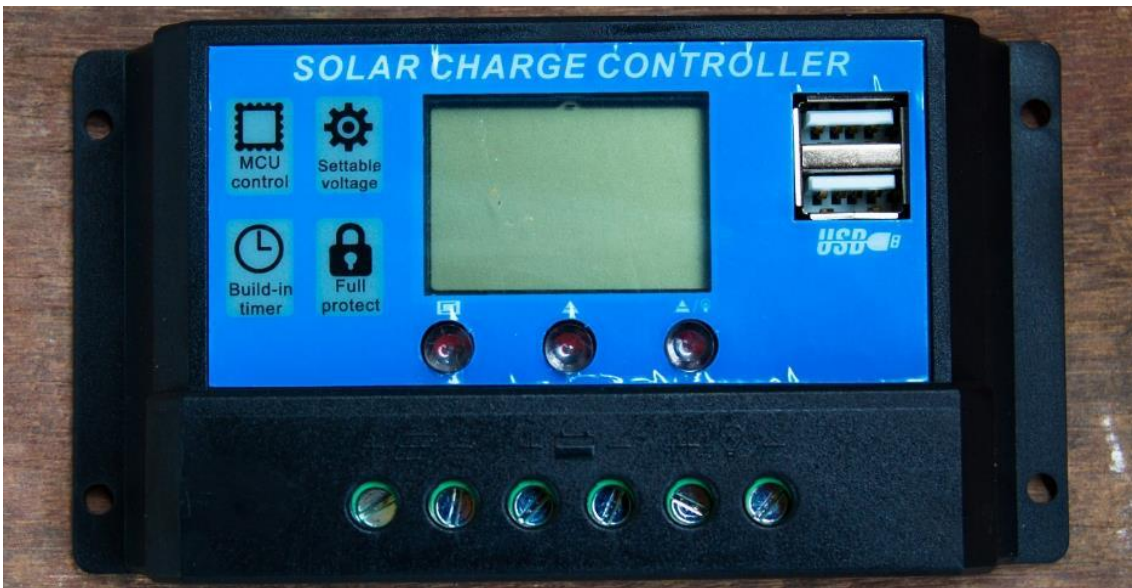
Figure 27. New solar charge controller (June 2019)
