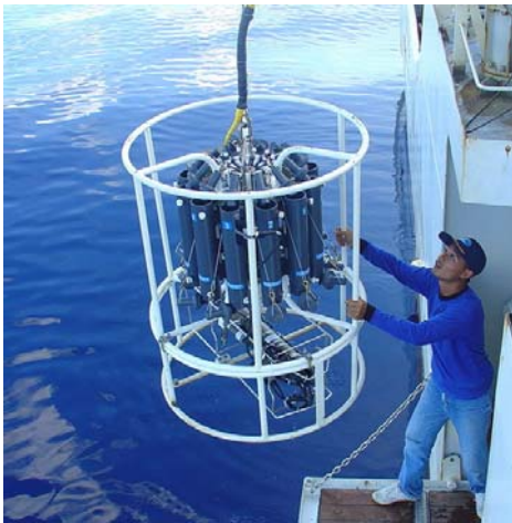
Fig. 1 Deploying of ICTD
